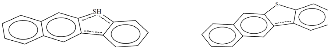
Figure 2: EPI Suite structural outputs using SMILES input (correct SMILES; left side image) and input of CAS number (use of EPI Suite SMILES database to retrieve SMILES, missing aromaticity in thiophene ring, right side image)
