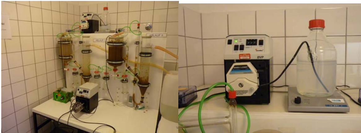
Figure 75: Laboratory sewage treatment plant day 21 end with 5 mg/L TiO 2 (left) and dosage of the TiO 2 suspension (detail) (right).
