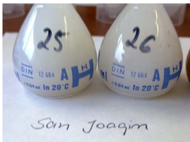
Figure 17: SRM 2709a after digestion. The white dispersion is centrifuged prior to analysis.
