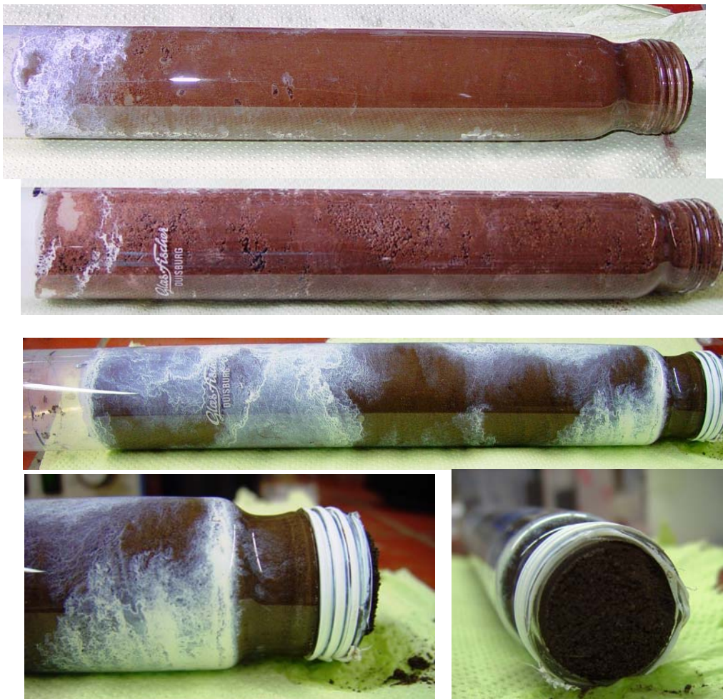
Figure 95: Soil columns after the test, before they were differentiated in different segments. Treated with UV Titan M262 – soil column filed with soil A01 (top), A06 (middle) and A04 (bottom).
