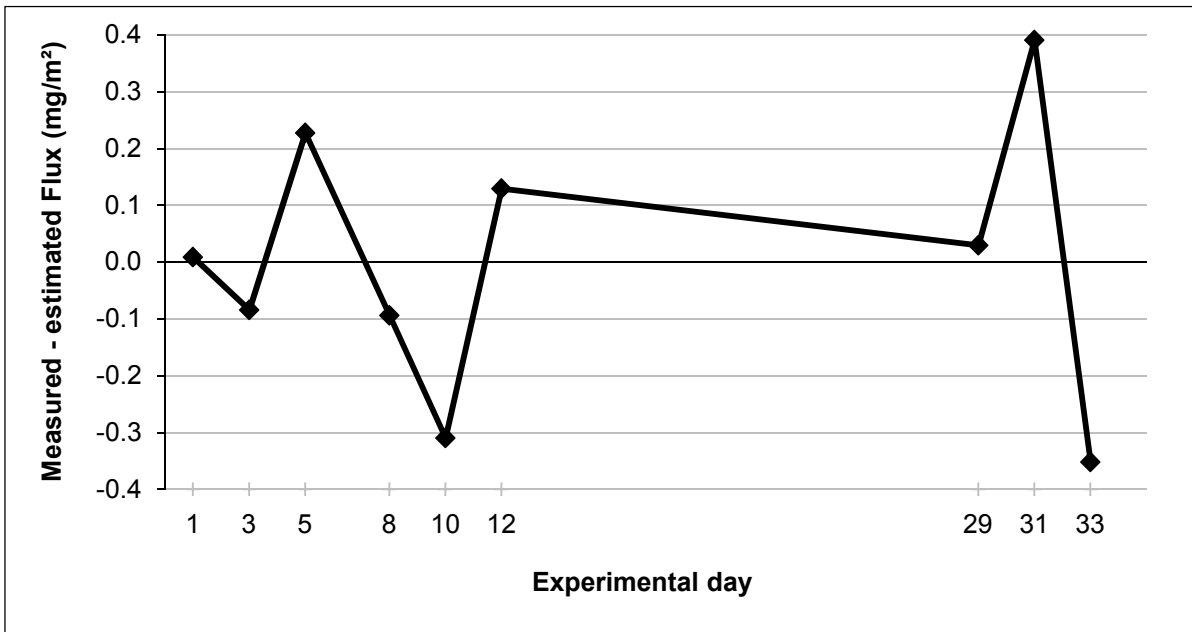
Figure 26: Deviation between measured and estimated Flux of analytical model (biocide: OIT, long-term test: OECD TG107 modified)
