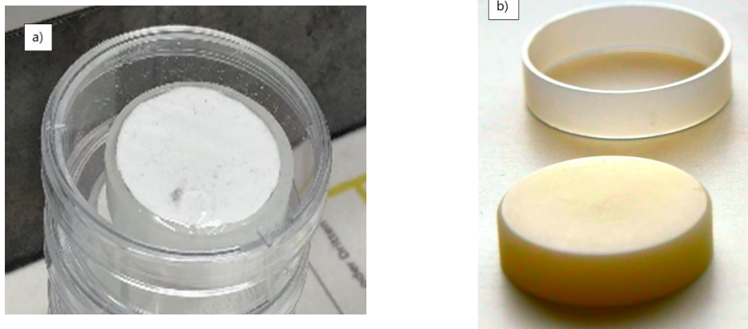
Fig. 2: a) Counting source, consisting of plastic disc, fixing ring and filter paper with precipitate and Mylar ® film, in a Petri dish; b) Plastic disc and fixing ring.
