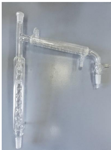
Fig. 1: Parts of the distillation apparatus: Vigreux column and Liebig condenser
